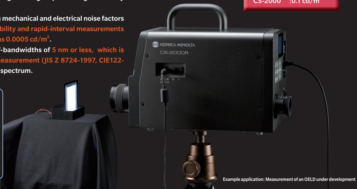
Example application: Measurement of an OLED under development
