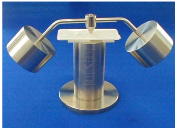
BPT-01 on Test Sample supported by BPA-01
