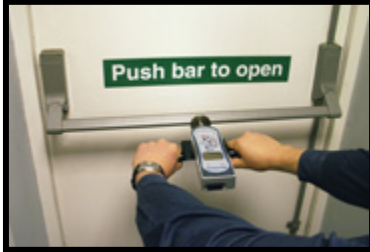
Gripping Cradle (in use at left): Enables comfortable 2-handed operation for testing push/pull loads
