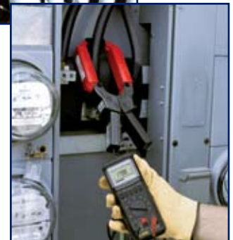
Model JM810A measuring current on a main branch circuit.
