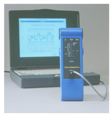
System FD 3 is used as a automatic dosimeter for exposure measurements where large variations of local magnetic fields occur in a space or over time. The dosimeter is loaded from a personal computer (PC) with measurement interval and mode parameters, date and time, location and contact person.
