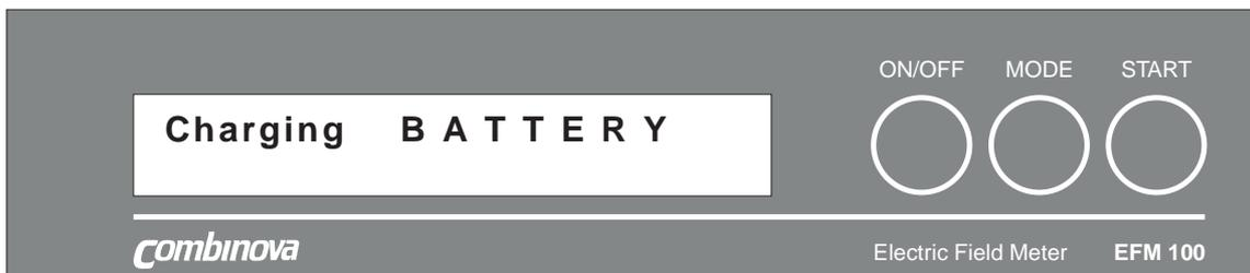
During charging, the battery voltage is constantly checked against different limits by the microprocessor to decide if the charging is working properly.
