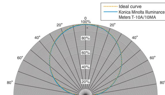
Since the brightness at the measurement plane is proportional to the cosine of the angle at which the light is incident, the response of the receptor must also be proportional to the cosine of the incidence angle. For Konica Minolta Illuminance Meters T-10A/10MA, the cosine response  $f_2$  is within 3%. The graph above shows the cosine correction characteristics of Konica Minolta Illuminance Meters T-10A/10MA.
