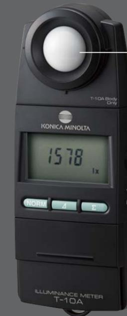
Receptor diffuser window: Ø 25 mm
