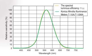
Ideally, the relative spectral responsivity of the illuminance meter should match V ( $\lambda$ ) of the human eye for photopic vision. As shown in the graph above, the relative spectral responsivity of Konica Minolta Illuminance Meters T-10A/10MA is within 6% (f1') of the CIE spectral luminous efficiency V ( $\lambda$ ).
