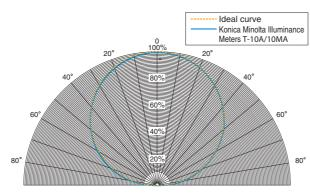
Since the brightness at the measurement plane is proportional to the cosine of the angle at which the light is incident, the response of the receptor must also be proportional to the cosine of the incidence angle For Konica Minolta Illuminance Meters T-10A/10MA, the cosine response f2 is within 3%.
