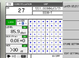
Spectral Display, OFDM 64QAM and Delay Profile Screens
