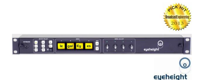
The LegalEyes is a full-featured A/V legalizer system. This instrument accepts SD/HD SDI sources, legalizes video and audio levels (including Loudness) and outputs a corrected SDI feed for use in downstream processes. It supports RGB, Composite (PAL, NTSC 7.5IRE setup and NTSC 0 setup), simultaneous Composite + RGB and YCbCr gamut correction.
