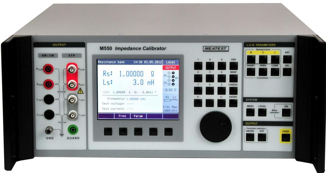
Basic applicable frequency range is from 20 Hz to 1 MHz in coaxial mode, and to 100 kHz in non-coaxial mode. Calibration memory contains both complex parameters of partial standards. The calibration values can be displayed in wide range of frequently used pairs of complex impedance and admittance. Either parallel or series equivalent model can be selected. The calibrator is equipped with reference positions OPEN and SHORT terminals for easy elimination of test cables influence.
