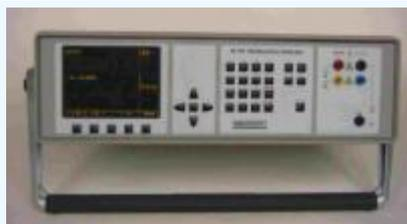
Multifunction calibrator M-140i is calibrator, determined mainly as standard of electric quantities in calibration laboratories. It can be used for calibration of electrical quantity meters from the field of voltage and current.
