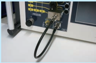
Check CDN line out.
