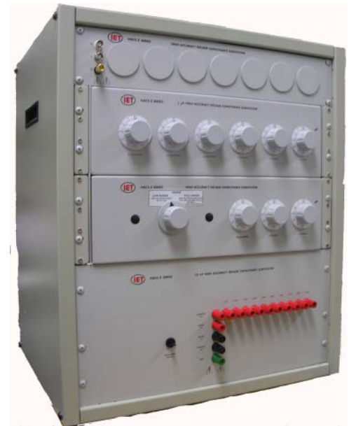
HACS-Z-10E-1pF 1 pF - 11,111.111 11 \mu F 1000 \mu F decade employs binding posts
