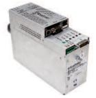
The MNX Series is designed to power grounded cathode X-ray tubes from a variety of well known manufacturers. It features a 0 to 50kV high voltage output, and up to 2mA of emission current limited to 50 Watts, operating from a +24Vdc input. The ground referenced low noise dc filament supply operates between 0.3 and 3.5 amps.
