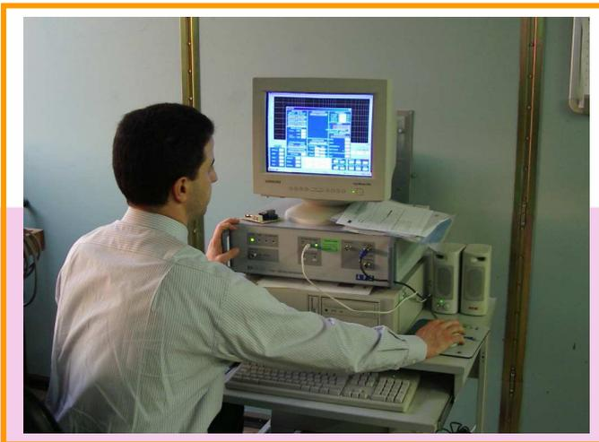
All information collected by the AFJ CL55C during the test, are displayed in real time on the PC screen, divided into a number of windows corresponding to the number of internal RF channels.
