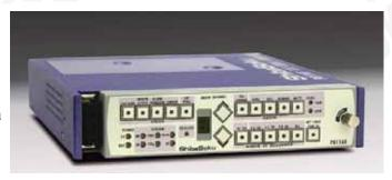
well as a function that allows you to check audio information. It also allows for superposition of the characters (logo and telop) that indicate sending and receiving stations or a program material name, etc.
